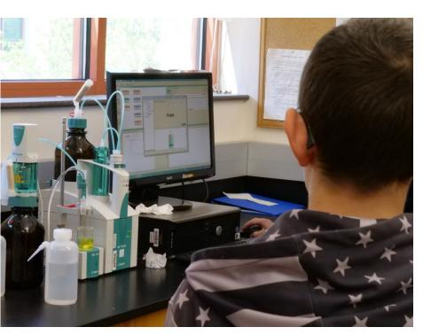
Cade observing the Metrohm automated titrator operated by Dustin Baca measuring alkalinity.
