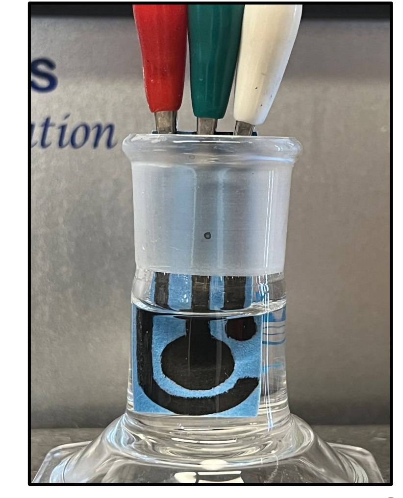
Paper-based Electrochemical Sensor connected to potentiostat
